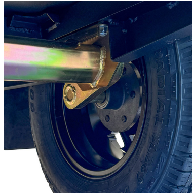
AL-KO IRS 80mm 800kg suspension.
