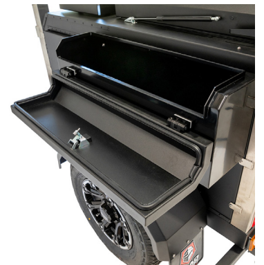
Rubber bulb seals around all openings.
